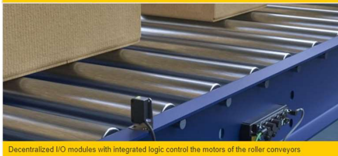
Decentralized I/O modules with integrated logic control the motors of the roller conveyors
